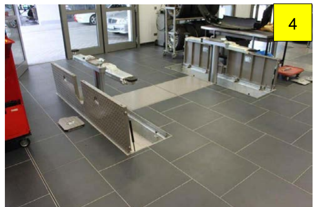
4 Raise the lift until it is above the top edge of the opened lids (lifting height approx. 1 m).
