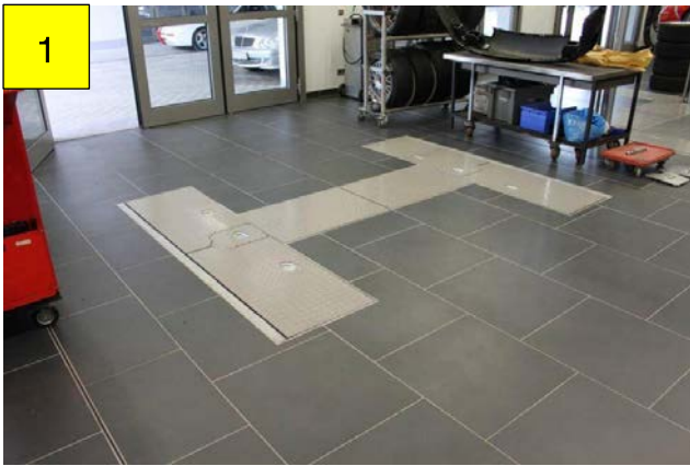
1 Lift with hinged-lid frame, fully flush with the floor.
