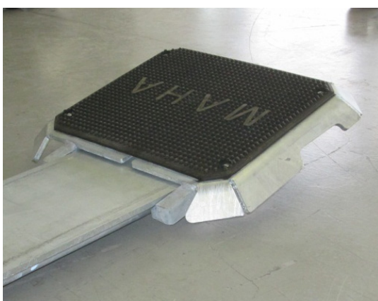
Flat head support not locked
